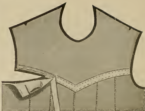
Fig. 159. Attaching Yoke to Front
